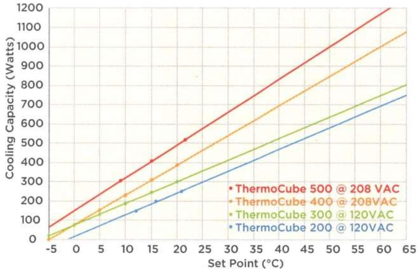
Note - Cooling Capacity will vary with configuration
