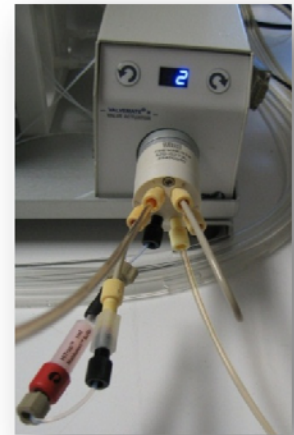
Figure 3: VALVEMATE II PEEK valve - Pos 1: access to transfer tubing - Pos 2: access to HiTrap™ column
