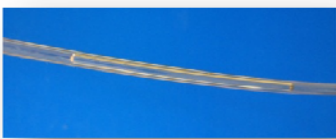
Figure 5: Radel R Tubing Showing Intact Air Gap
