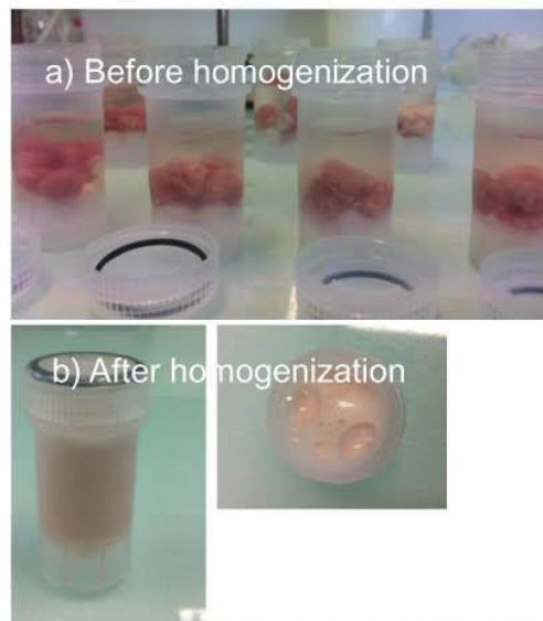
Figure 1: 6 mouse brains in a 15mL Precellys® tube before (a) and after (b) homogenization using the Precellys® Evolution.
